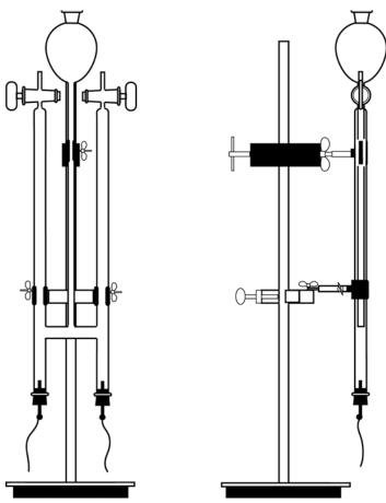
glass tubes are connected to a 9-volt battery or power supply via connector cords.
