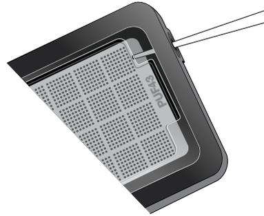
It is important that the syringe tip is in front of the array when filling the case with immersion fluid.
