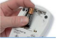
Open the battery compartment on the back of the meter.
