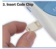
Make sure the meter is off. With the code number facing up, insert the code chip into the code chip slot until it snaps into place.
