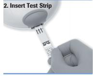
Slide the test strip into the test strip guide in the direction of the arrows until
