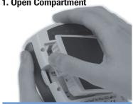
Press the release tab on the battery cover on the back of the meter. Slide the battery cover off.
