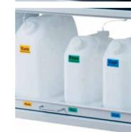
9 The integrated bench includes containers for wash and rinse solutions and for solid and liquid waste (ability to pump waste out to drain).
