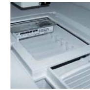
7 Strip tray (8 positions) or calibrator strips and/or curve control strips.
