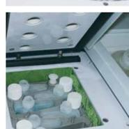
4 Sample diluent (6 bottles) and dilution plates (2 x 96 wells) for onboard dilution of samples.
