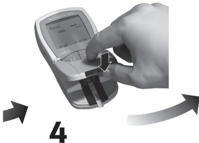
Start measurement by closing the measurement chamber flap
