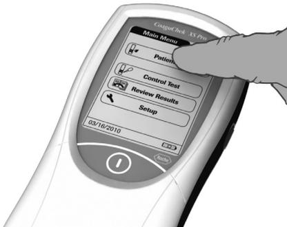
You can open any displayed function by touching (or tapping) the button for it with your finger (or a special pen for this purpose). “Tap” means: Touch the button, then remove your finger from the touchscreen. The next screen appears once you remove your finger.
