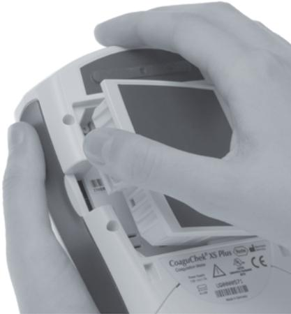
**1** With the meter turned off, press the battery compartment cover release tab and slide the cover off.
