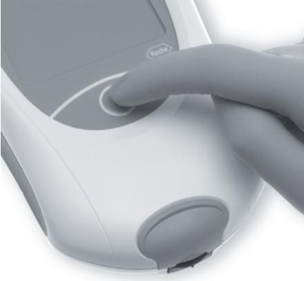
**10** Place the meter on a level, vibration-free surface, or hold it in your hand so it is roughly horizontal. Turn the meter on by pressing the ON/OFF button
