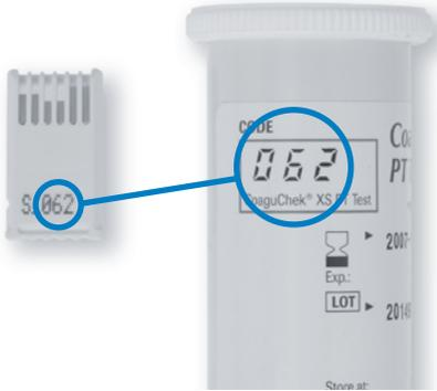
**2** Always make sure that the number on the code chip matches the number on the label of the test strip container.
