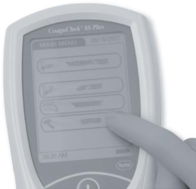
You can call up any displayed function by touching the screen prompt for it with your finger (or a special pen for this purpose). Touch the screen lightly, holding until the prompt is selected.
