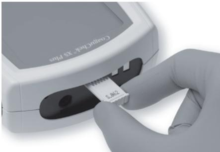
**3** Slide the new code chip into the code chip slot (as shown) until you feel it snap into place.
