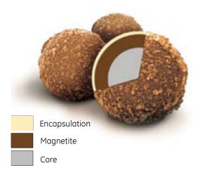
Sera-Mag Magnetic Particles feature a single layer of magnetite but with the same cauliflower-like surface of the SpeedBeads.
