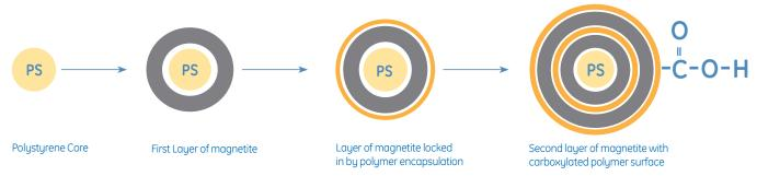
Sera-Mag SpeedBead Carboxylate-Modified Magnetic Particles feature carboxylic groups on the surface that permit easy covalent coupling using simple carbodiimide chemistry.
