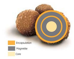
This SEM image shows the cauliflower-like surface of the Sera-Mag SpeedBeads which dramatically increases the overall surface area available for binding. Sera-Mag SpeedBeads also have a second layer of magnetite within the particle, resulting in a 2x faster increase in speed in response to a magnetic field.
