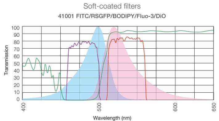
Superior transmission efficiencies are observed using hard-coated filters on the EVOS instruments, compared to soft-coated filters. Excitation filter (purple), emission filter (red), dichroic mirror (green); Invitrogen™ Alexa Fluor™ 488 excitation (blue), 488 emission (pink).
