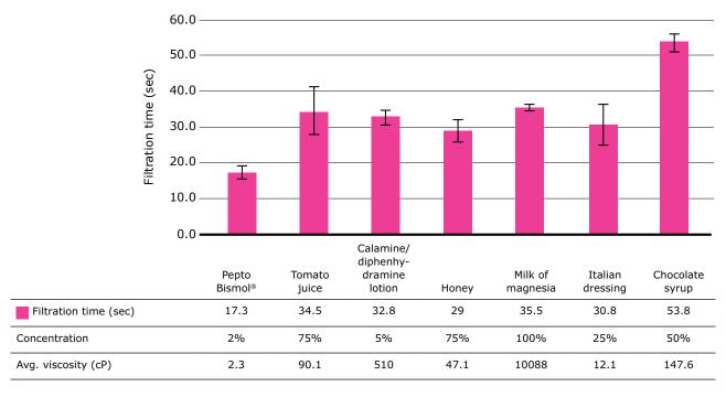
Hard to filter? No More! Efficient filtration of viscous samples using the Samplicity® filtration system with 0.45  $\mu$ m PVDF Millex Samplicity® Filters. Filtration times for 1 mL of indicated samples are shown. Results represent the average of four filtrations, and error bars represent standard deviation.
