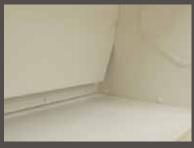
Downflow Rear Baffle - Baffle is biased to the bottom, drawing fumes downward away from the user. Exhaust air exits the fume hood at work surface level preventing lighter-than-air fumes from rising up into the face of the user while effectively capturing and removing heavier-than-air fumes as well. Baffle actuators and controls not required.
