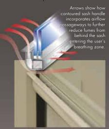
Performance Sash Handle - Incorporates an airfoil design and provides improved airflow along the lower edge of the sash to prevent turbulence from resulting in a hazardous release. Powder coated stainless steel handle incorporates an airfoil design and provides improved airflow along the lower edge of the sash to prevent turbulence from resulting in a hazardous release.
