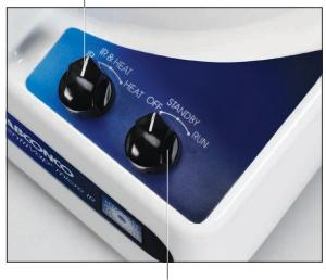
Run Mode Selector. Use to select Off, Standby (preheat) or Run mode.
