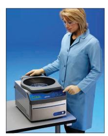
CentriVap Vacuum Concentrators, such as the Acid-Resistant CentriVap shown above, process up to 132 samples at once.
