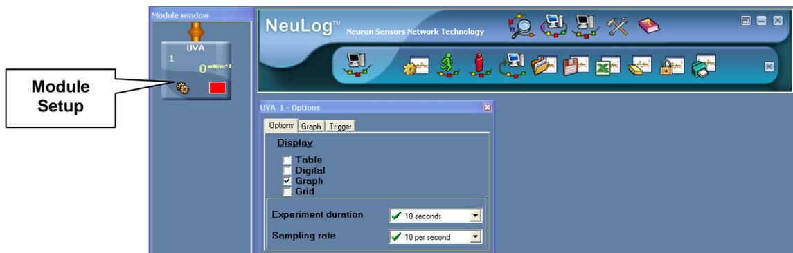
This procedure downloads the measurement conditions to the sensor and these are stored in its memory.
