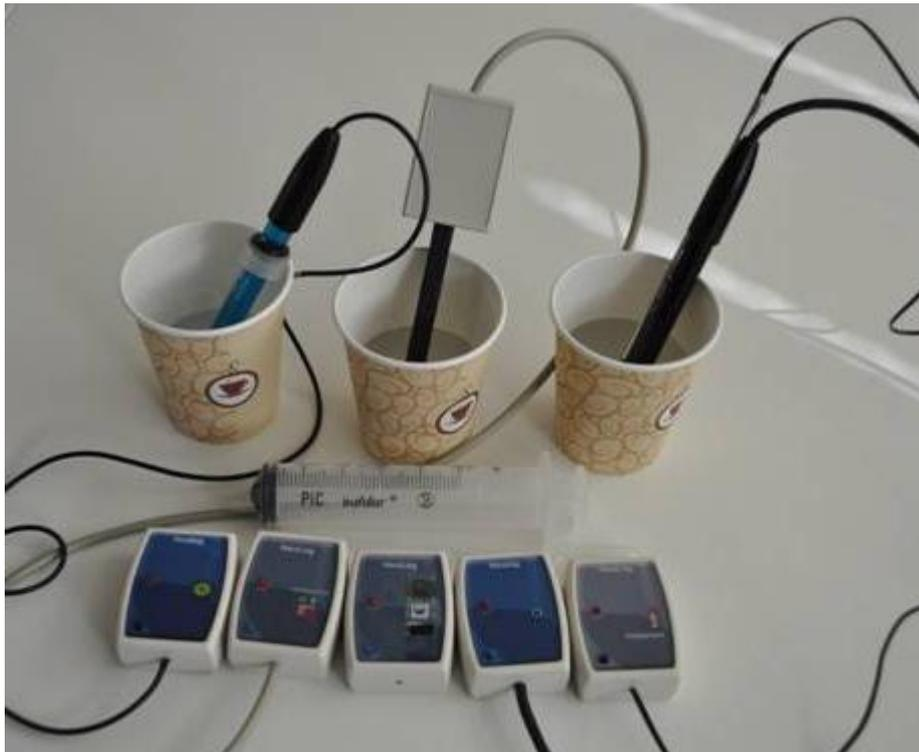
17. Since sensors may interfere with each other, divide the first sample of water into three cups. There should be enough water so that all the sensitive parts of the sensors are immersed.
