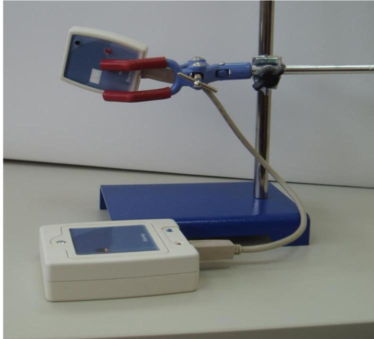
You will have to change the sensor module for each measurement, i.e. start with the Light Sensor, perform a measurement, then switch to the UVA Sensor and then to the UVB Sensor.
