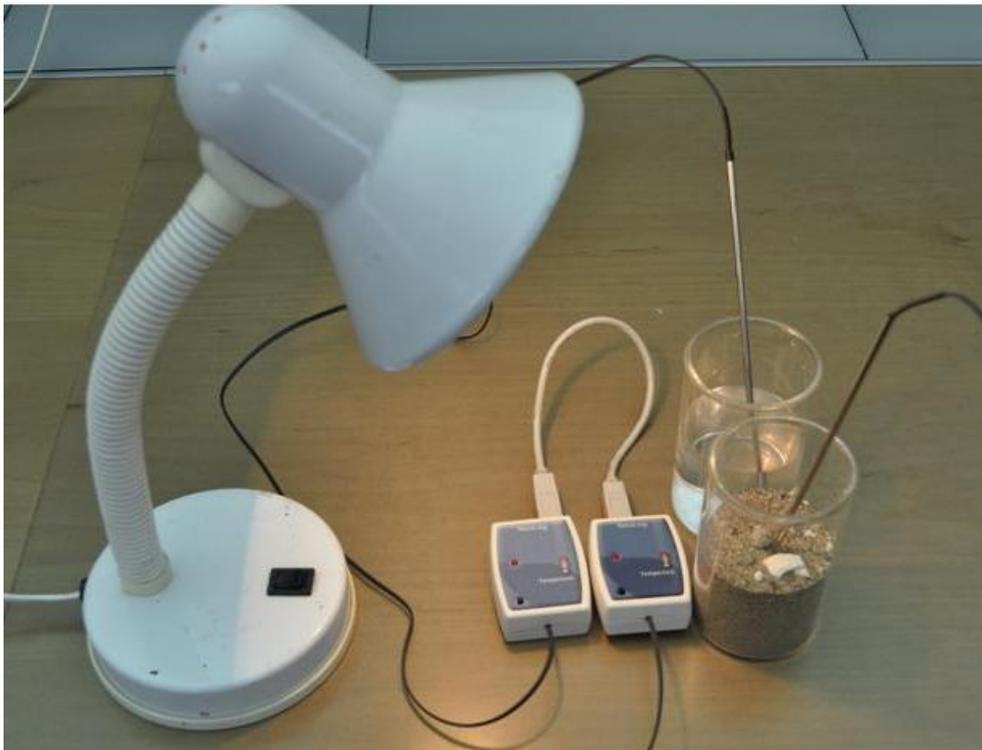
1. Fill one beaker with 300 mL dry sand at room temperature.
