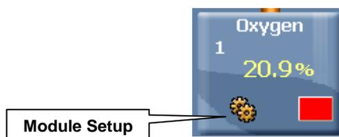
12. Whether you used the Load Configuration function or not, click on the 'Calibration' icon
