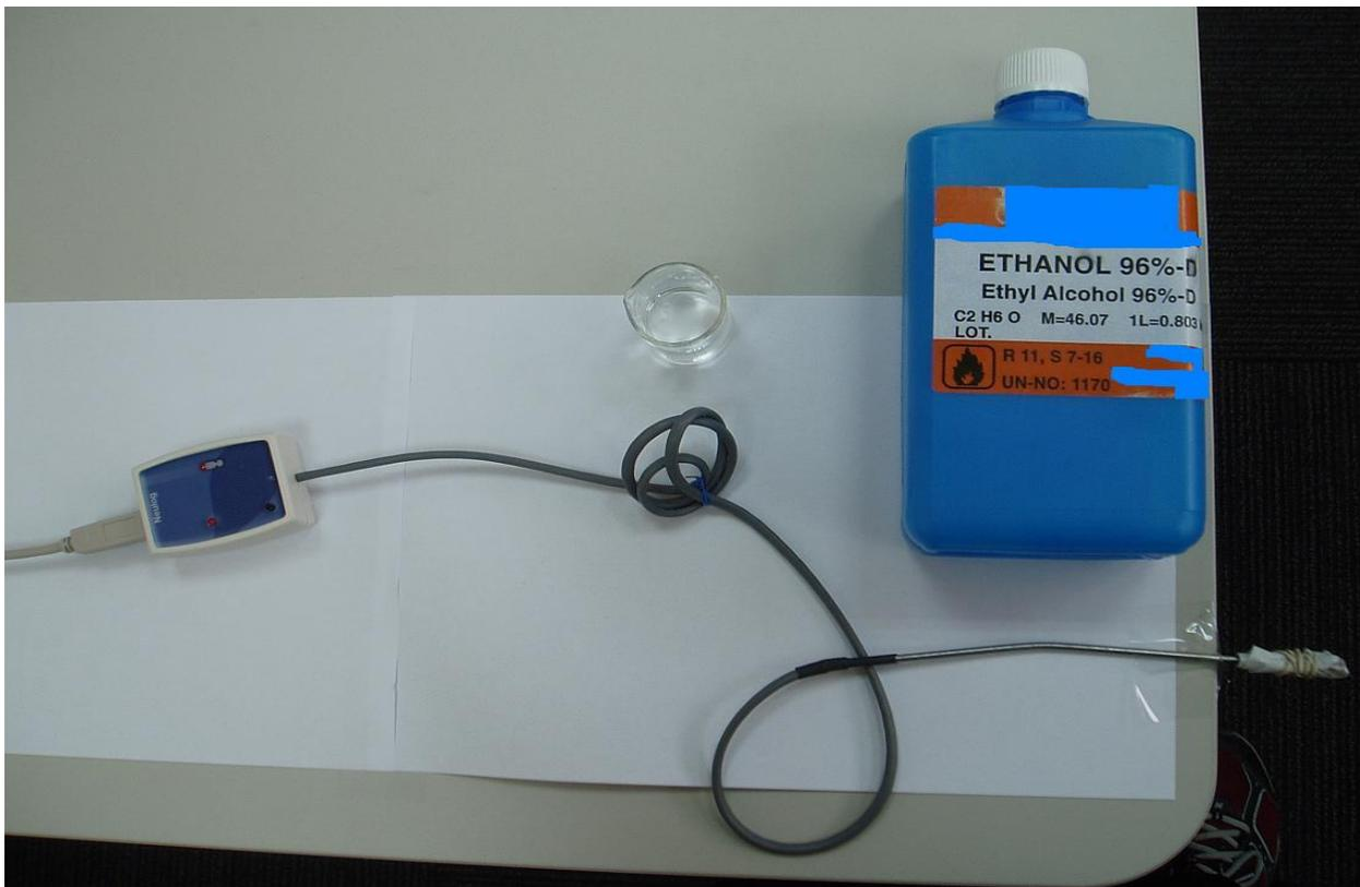
1. Wrap the tips of two temperature sensors with a small piece of cotton and secure it with a small rubber band. Wrap the cotton evenly.
