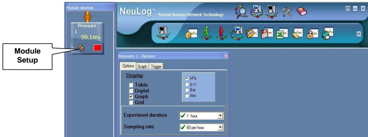
This procedure downloads the measurement conditions to the sensor and these are stored in its memory.
