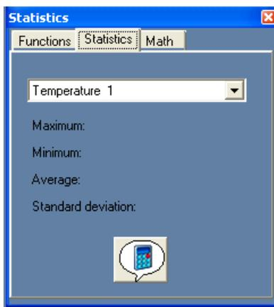
22. Select the Temperature Sensor from the scroll down menu in the opened window. Click the 'Calculate Statistics' icon
