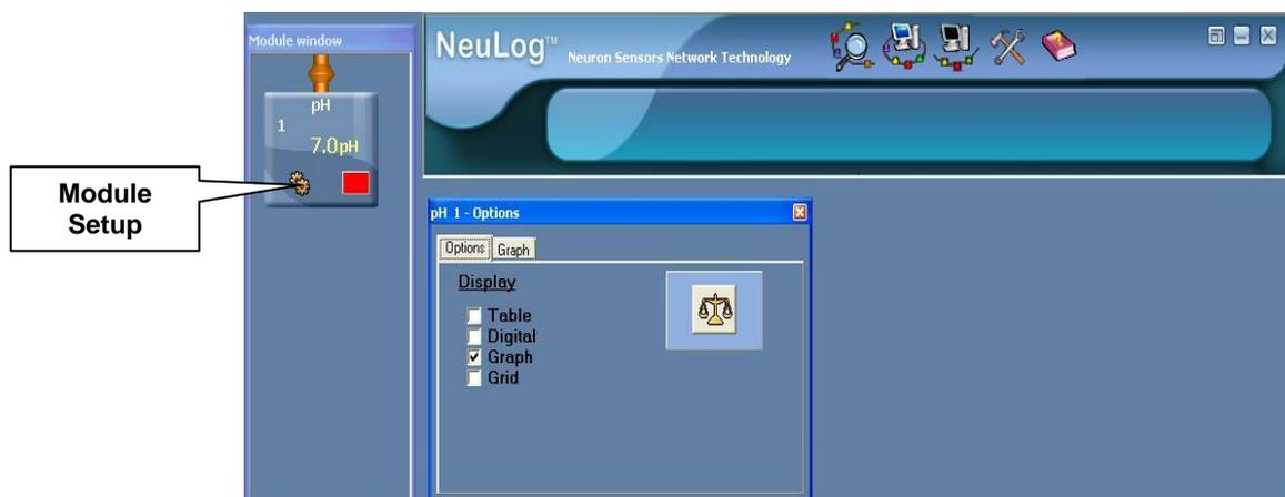
18. Click on the 'Calibration' icon
