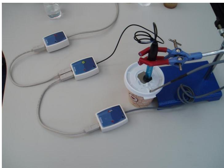
2. Take the plastic cover of a coffee cup and make two holes one for the pH and the other for the Temperature Sensor (see picture).
