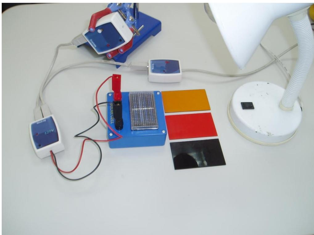
2. Connect the red lead of the Voltage Sensor
