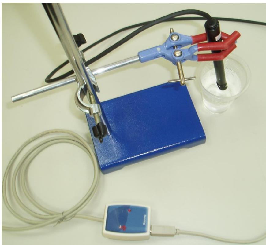
2. Add 70 ml of distilled water to a clean 100-ml cup and put it in front of the sensor.
