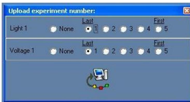
40. Upload the measurements to your computer. The measurements were saved in the sensor's memory. Select the two radio buttons next to the number 5 (one for each sensor). This way, you are selecting the first measurements to be uploaded.
