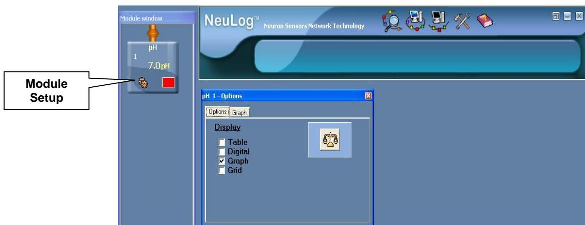
18. Click on the 'Calibration' icon
