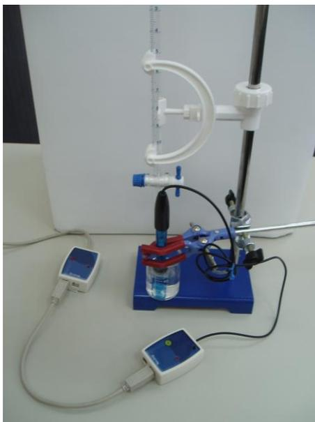
2. Put the pH Sensor in the tube holder on the stand and introduce it in water stirring carefully to remove the soaking solution.
