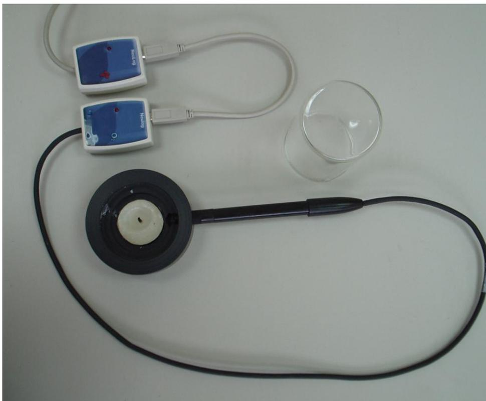
1. Remove the rubber protection from the Oxygen Sensor's cap. Unscrew the cap, fill half of it with the included liquid and then close it.
