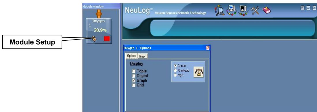
14. Verify the mode is "% in liquid". Click the 'Calibration' icon
