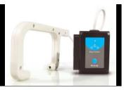
The NeuLog drop counter sensor uses an infrared beam which passes between the two endpoints of the sensor probe to determine drops. As liquid falls through the infrared beam infrared light is scattered and not detected at the infrared detector on the opposing side. Regardless of the liquids opacity or color, the infrared light will bend away from the detector. Every time there is a break in the infrared beam, a drop is counted at up to 100 samples per second.
