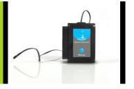
Your surface temperature sensor needs to be connected to a WIFI-201 module. The WIFI-201 module will create a closed NeuLog wifi network which will stream the NeuLog data to a device of your choosing. Once your device is wirelessly connected to the NeuLog network you can run experiments and collect data through a browser of your choosing.
