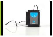
The surface temperature uses a partially exposed thermistor to rapidly detect temperature changes of surfaces compared to other thermometers which require the outer protective layer to change temperatures first. Temperature changes in the thermistor's wires act as variable resistance which is directly measured. When more heat is present the wires are slowed at a greater rate. The amount of resistance is rapidly measured and converted into a temperature readout almost instantaneously.
