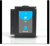
Your UVB sensor needs to be connected to a WIFI-201 module. The WIFI-201 module will create a closed NeuLog wifi network which will stream the NeuLog data to a device of your choosing. Once your device is wirelessly connected to the NeuLog network you can run experiments and collect data through a browser of your choosing.
