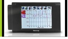
Along with all of the buttons located across the top of the screen, you can directly click on each individual sensor to change the experimental parameters such as the units to collect in.
