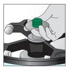
Push center button to remove rotor
