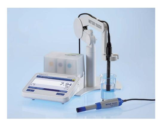
The SevenExcellence S900 benchtop instrument provides customers a premium benchtop solution to measure dissolved oxygen (D0) in aqueous media. Whether you measure D0 using the traditional polarographic or the new digital optical dissolved oxygen technology (OptiOx), the S900 guarantees precise and highly reproducible results.
