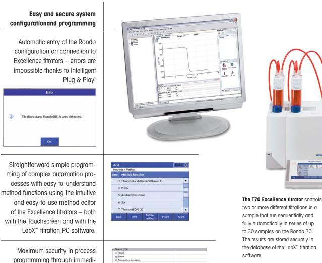
Maximum security in process programming through immediate plausibility checks of method sequences: only a correct method is saved.
